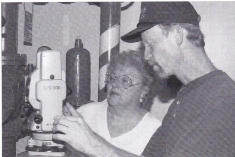
NIMA's Mark Belrose shows Madeline Akronowitz features of a Total Station, an electronic theodolite.
